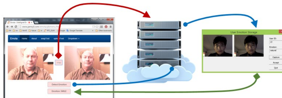
Figure 5: transfer of captured images to a server application, and the return of a detected emotion.
